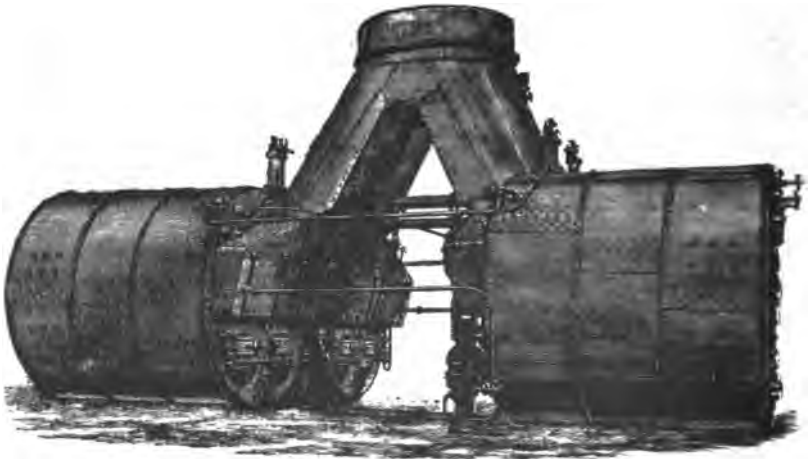
FIG. 33.—SETTING AND CONNECTION OF SCOTCH BOILERS.
